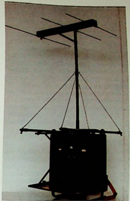
Yagi-antenne in meetopstelling (1934).
